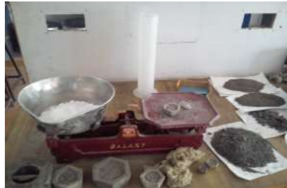
Figure. 2. Taking the weight of mixture of cement
