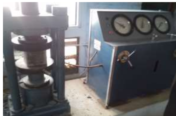
Figure. 4. Testing machine of blocks
